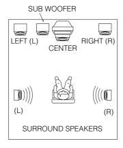
If possible, mount the surround speakers on the walls to the sides of the viewing area, 2-3 feet above seated viewers, firing straight across at each other.
